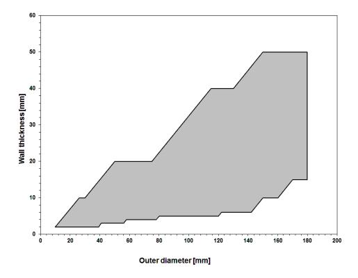
Dimensions in several strength and hardness conditions for seamless tubes are available on request.
